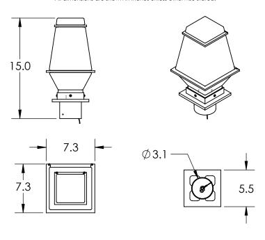
Mounting Method: Mounts Directly to Post
